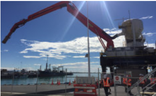
BULK MATERIAL AND LIVE STOCKS MANIPULATOR Working radius up to 44m.
